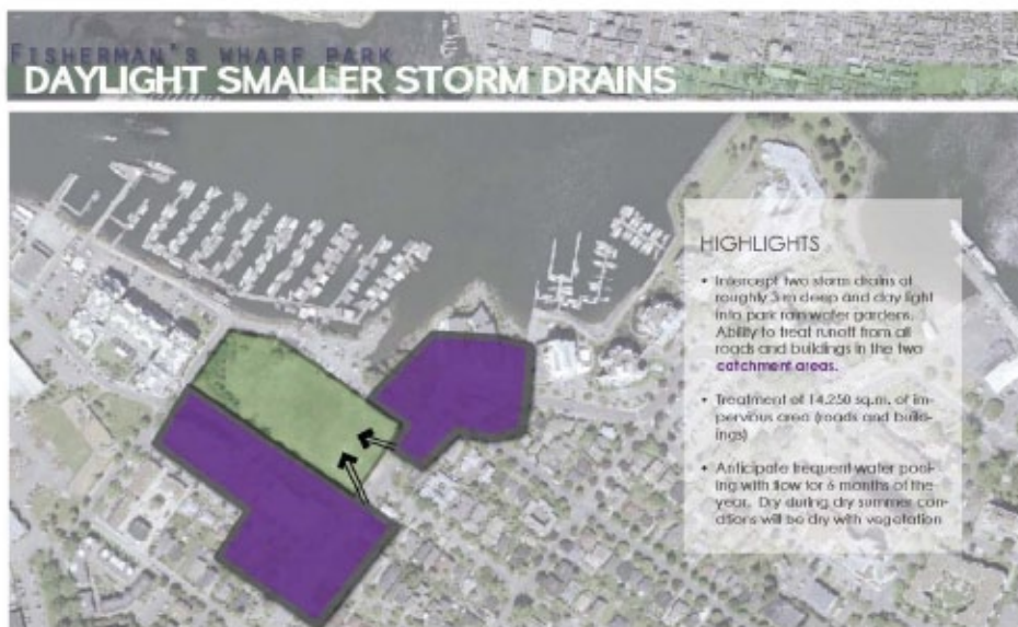
Figure 3. Proposal to intercept runoff from two adjacent catchment areas
