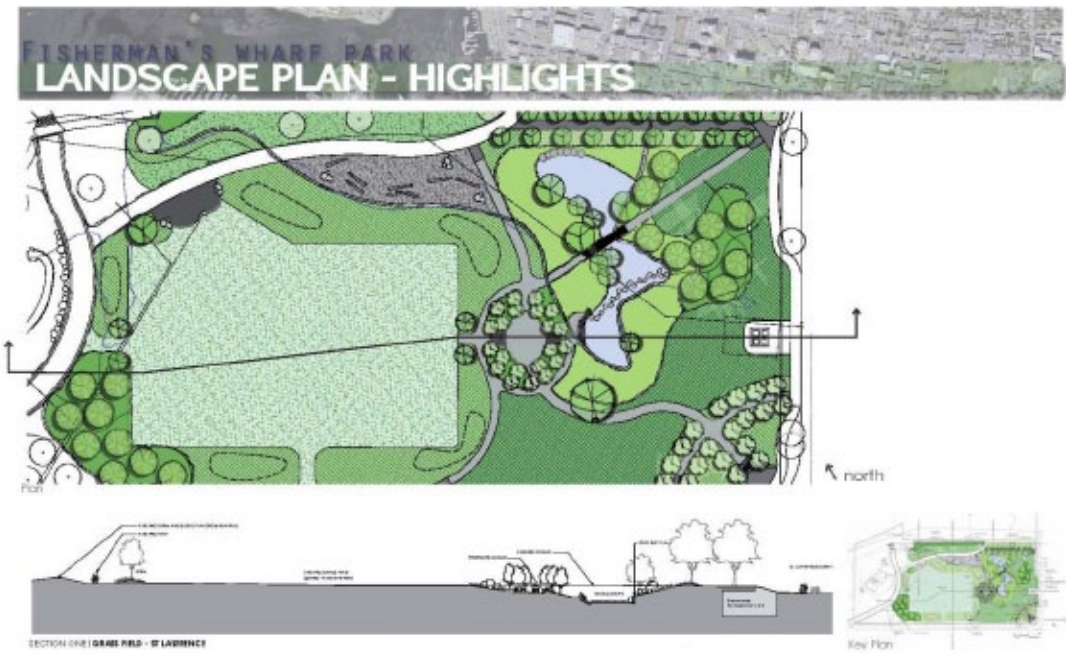
Figure 6. Landscape plan with section through park and rain garden
