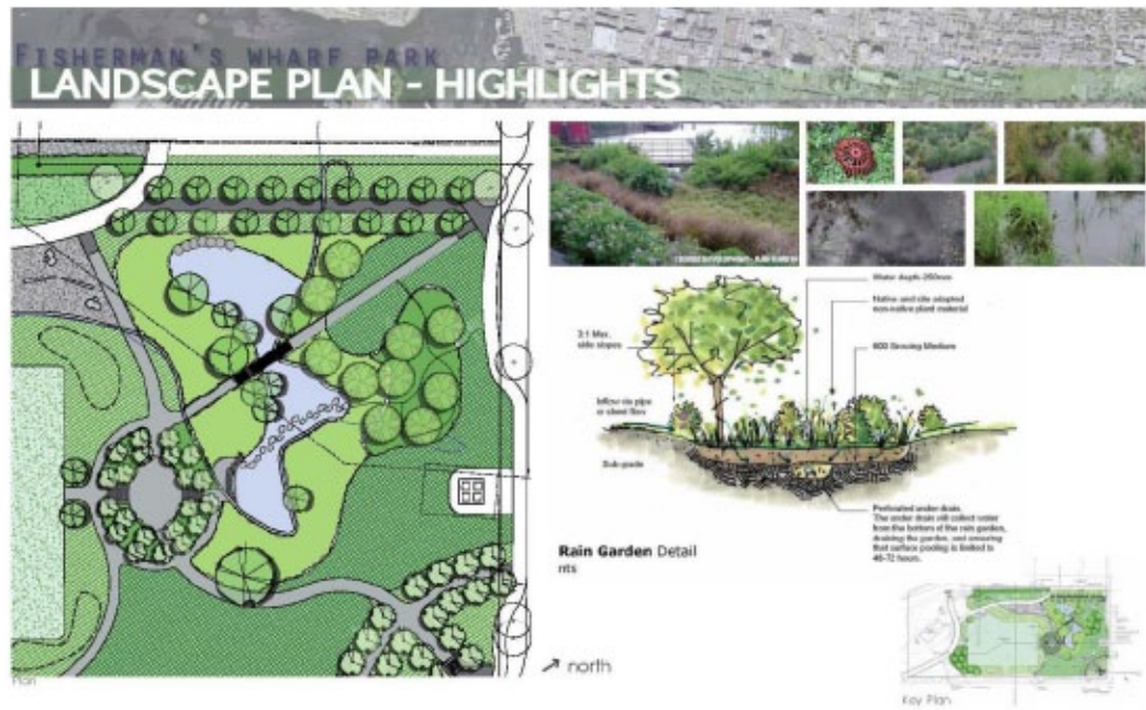
Figure 8. Detailed design of the rain garden
